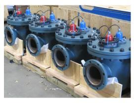
Anodes can be installed in a strainer (shown above), in an anode housing, in a tee, in the sea chest, etc.
